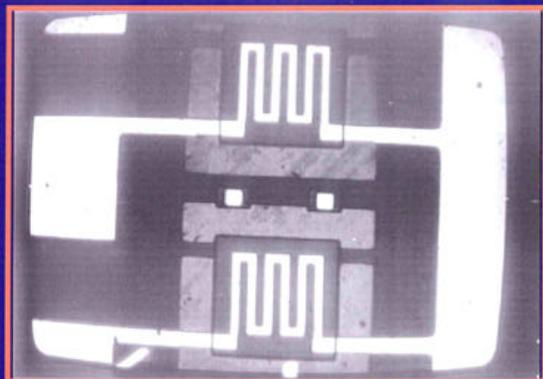
1000 Å Ti deposited over 0.5 μm SiO<sub>2</sub> membrane suspended over 1 μm air gap. IR sensitivity 1mV/μW
