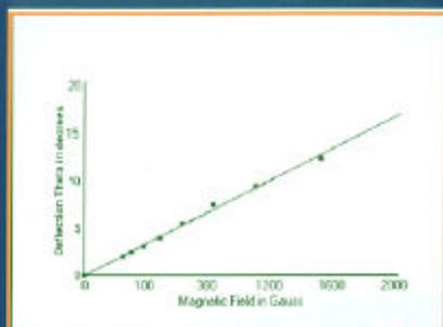
Si unbalanced torque arm is coated with Cobalt for H-field sensing.
