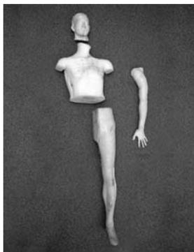
Figure 7 DOE's 'Human <sup>241</sup>Am Phantom' incorporating half of Case 0102's skeleton
