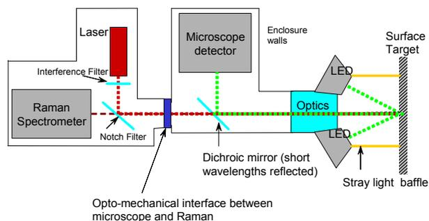
Figure 1. Basic Raman Microscope instrument configuration.
