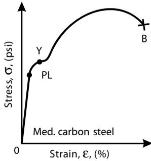
**Figure 2-8** Stress/strain curve for medium carbon steel
