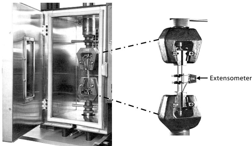
**Figure 2-6** Tensile test equipment and temperature chamber
