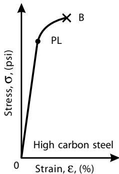
**Figure 2-10** Stress/strain curve for high carbon steel
