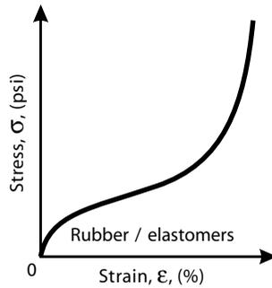
**Figure 2-12** Stress/strain curve for rubber or elastomeric materials
