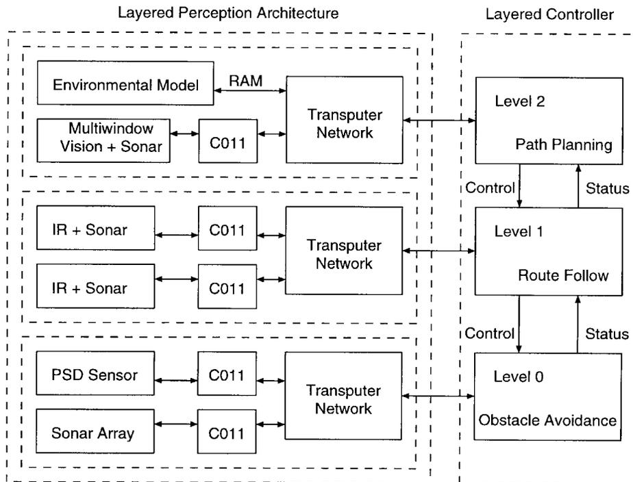
Fig. 3. A layered architecture for sensing [1].
