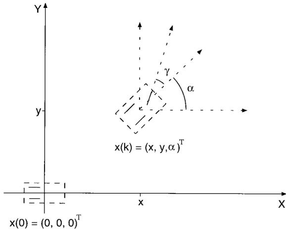
Fig. 2. AGV system geometry [11].
