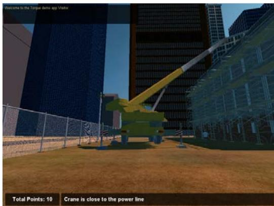
*FIG. 1: Point earning with an instructional message when a player correctly identifies that the mobile crane is too close to an overhead power line.*
