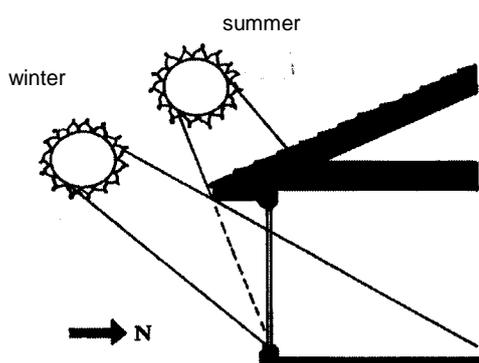
2.10 Overhangs shade a house from excessive solar gain in the summer, and allow sufficient sunlight to enter the building during winter months when the sun is lower.
