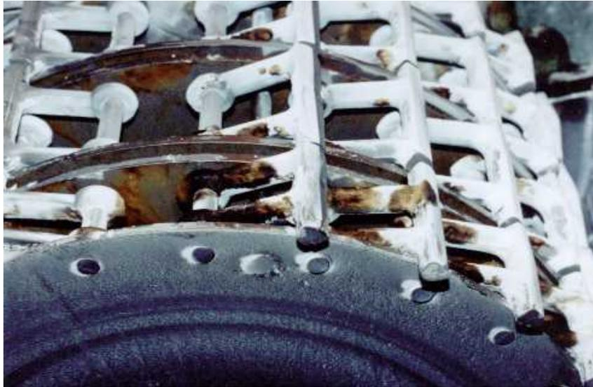
**Figure 1 Scorched hammers in a hammermill.**
