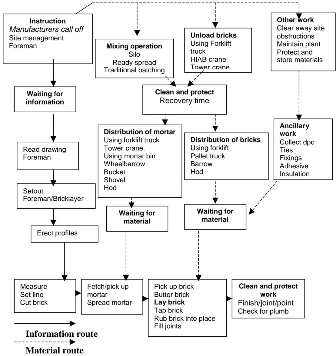
Figure 4 Brickwork production ‘as is’ process mapping
