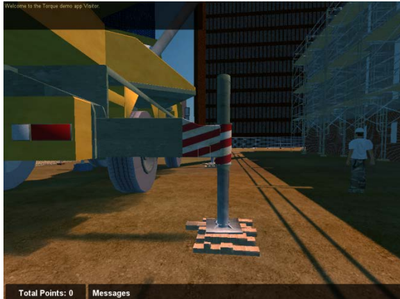
FIG.7: Collision-detection boundary for the crane makes the selection of wood blockings a challenge.
