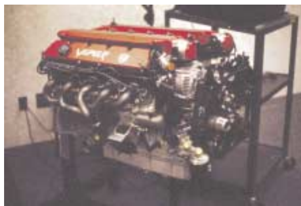
Viper V-10 engine with 400 honest horsepower, 450 ft-lbs of torque, and $16,500.
