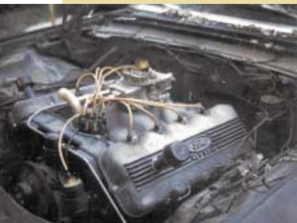
Ford 427 SOHC engine with overhead roller cam, hemi heads, four-bolt mains, forged-steel crank, and 600+ hp.
