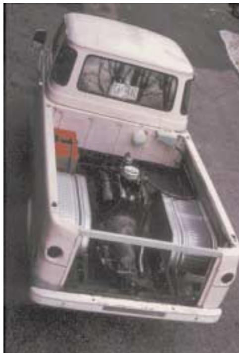
1963 Ford Econoline with rear-mounted 1972 Jeep power train.
