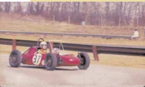
Formula Vee race car—VW running gear.
