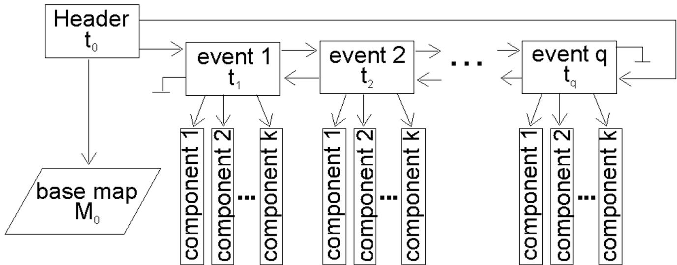
**Fig.5: Primary elements and the pointer structure of an ESTDM (Peuquet and Duan, 1995).**
