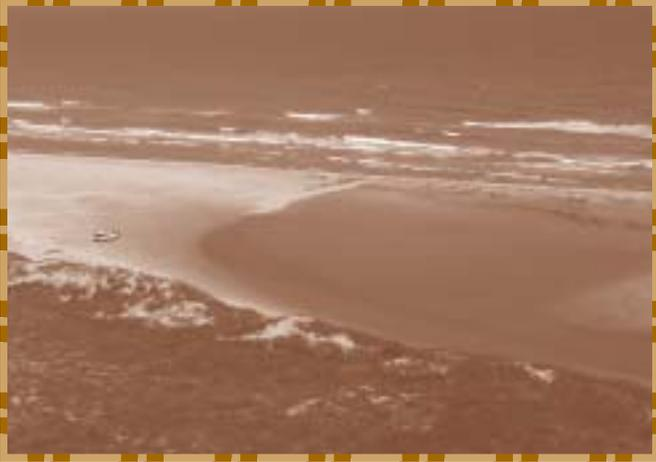
*For the first time in recent memory, the mouth of the Rio Grande became blocked with sediment during February 2001. Five months later, the IBWC dredged a 20-foot channel through the 440-foot sandbar.*
