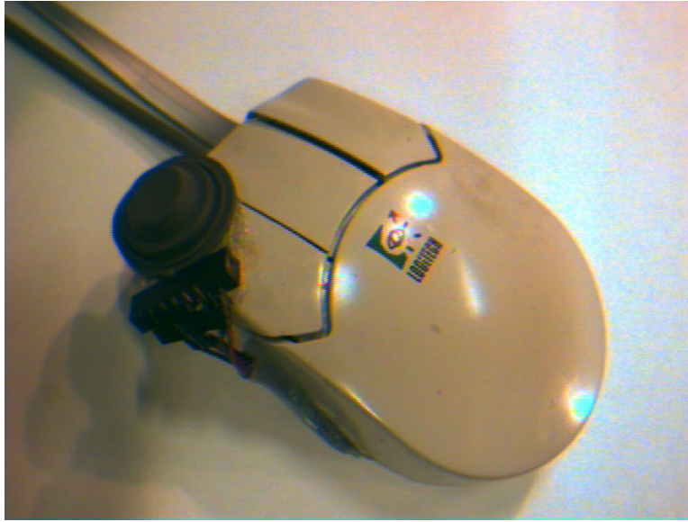
Figure 3-1: The sentic mouse uses a force sensor on the index button to measure the dynamic finger pressure of a user.
